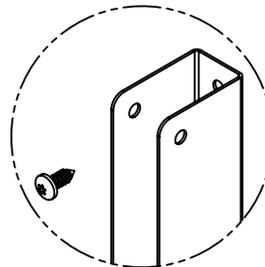
**C** Secure the continuous bracket to the pilasters using the #14 x 5/8" stainless screws provided.
