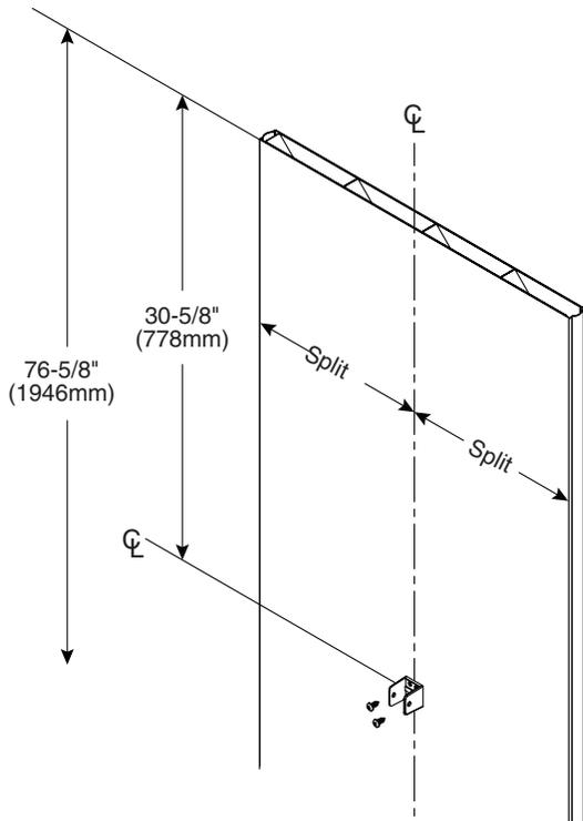
**A** **8' Ceiling:** Measure 30-5/8" (778mm) and 76-5/8" (1946mm) down from the top of each pilaster and place a mark on the pilaster split centerline.
