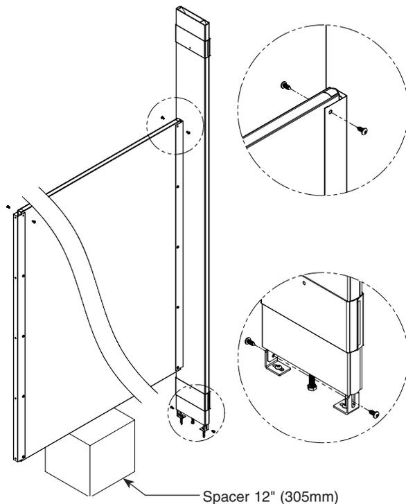
**D** Using the bracket as a template, drill Ø3/16" holes through the panel at each panel bracket hole. Secure the panel to the bracket using the #14 x 5/8" stainless screws provided.
