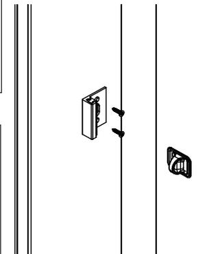
**E** Position the coat hook 36" (914mm) above finished floor (hook goes on the inside of compartment). Using the hook as a template, drill (2) Ø3/16" pilot holes through inside face of the pilaster only and secure with the #14 x 5/8" screws provided.
