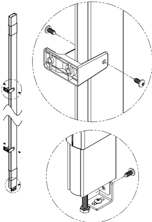
**C** Using the bracket as a template, drill Ø3/16" holes through the pilaster at each pilaster bracket hole. Secure the pilaster to the bracket using the #14 x 5/8" screws provided.
