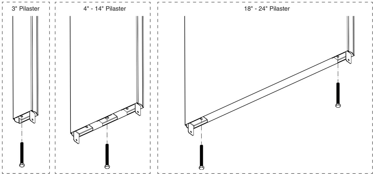
**A** Use leveling bolt(s) to adjust height of pilaster as indicated based on pilaster width.
