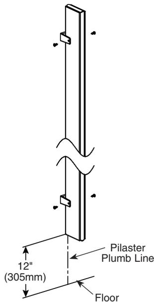
**Pilasters at Pilasters**
