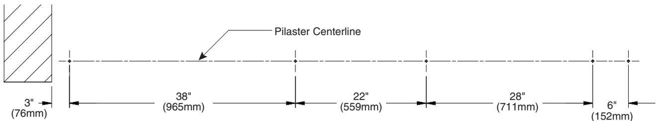
**B** Drill  $\text{\O}5/16"$  holes (min 2" [51mm] deep) into the floor and make sure the holes are free of dirt and debris.
