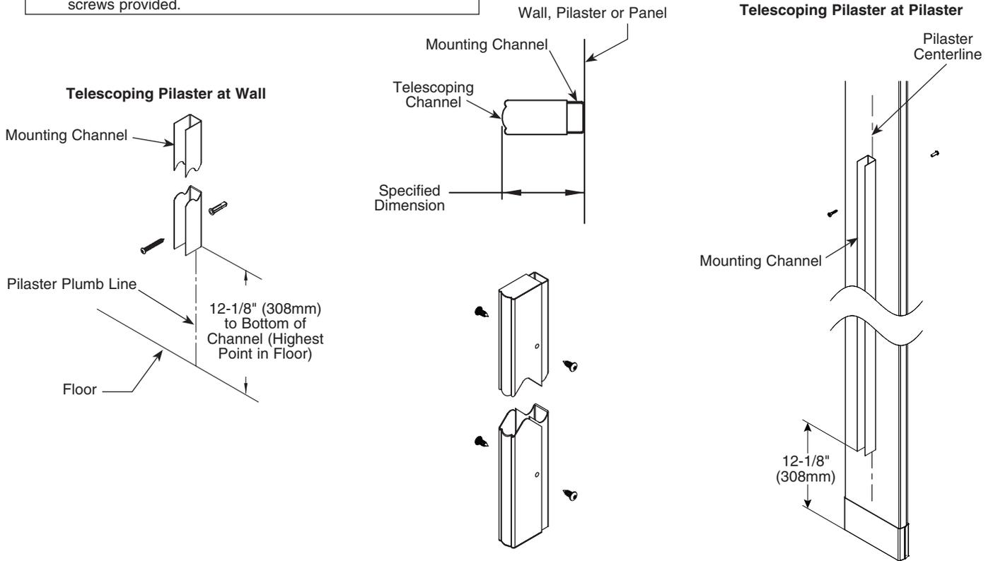
**6d Wall-Hung Pilasters (58") - Stirrup Brackets (Optional)**
