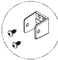
**C** Secure the stirrup brackets to the pilasters using the #14 x 5/8" screws provided.
