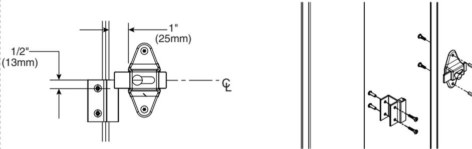
**B** With the door in the closed position, position the strike/keeper on the pilaster and align the top so it is 1/2" (13mm) above the bottom of the latch slide bar. Using the strike/keeper as a template, mark the hole locations and drill Ø1/4" holes through the pilaster. Secure the strike/keeper to the pilaster with the #10-24 x 3/4" barrel nuts and #10-24 x 1" shoulder screws provided.
