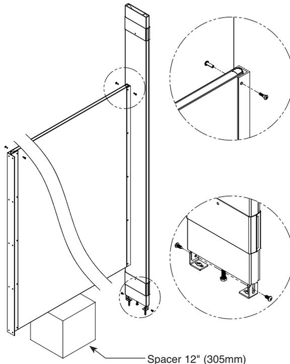
**D** Using the bracket as a template, drill Ø1/4" holes through the panel at each panel bracket hole. Secure the panel to the bracket using the #10-24 x 3/4" stainless barrel nuts and #10-24 x 3/4" stainless shoulder screws provided.
