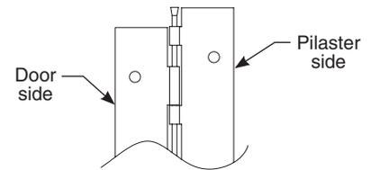
**A** Place a door on a 12" (305mm) spacer and set the door gaps. Standard hinge side gap is 9/32" (7mm).
