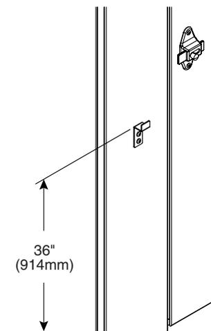
**E** Position the coat hook 36" (914mm) above finished floor (hook goes on the inside of compartment). Using the hook as a template, drill (2) Ø3/16" pilot holes through inside face of the pilaster only and secure with the #14 x 5/8" screws provided.
