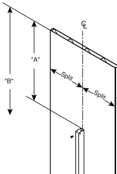
**A** **8' Ceiling:** Measure down from the top of the pilaster and place a mark on the pilaster centerline at dimensions "A" and "B" for the respective bracket (see table on left).
