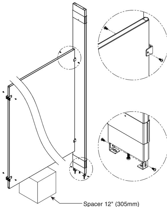
**D** Using the bracket as a template, drill Ø3/16" holes through the panel at each panel bracket hole. Secure the panel to the bracket using the #14 x 5/8" screws provided.
