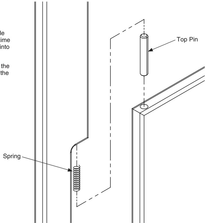
7. With the door in the desired "at rest" position, measure approximately 3" (76mm) down from the pilaster cutout and place a mark centered on the pilaster edge.
