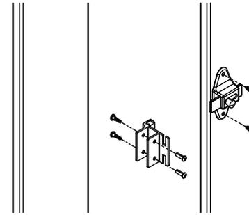
2. With the door in the closed position, place the strike/keeper on the pilaster and align the top so it is 1/4" (6mm) above the bottom of the latch slide bar. Using the strike/keeper as a template, mark the hole locations and drill Ø1/4" holes through the pilaster. Secure the strike/keeper to the pilaster with the #10-24 x 3/4" barrel nuts and #10-24 x 3/4" shoulder screws provided.
