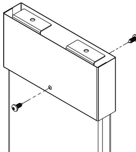
4. Using the hole in the bottom shoe as a template, drill a  $\text{Ø}1/4$ " hole through the pilaster. Secure the pilaster to the bottom shoe using the #10-24 x 3/4" barrel nut and #10-24 x 3/4" shoulder screw provided.
