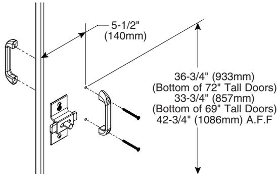
**D** Position the coat hook 36" (914mm) above finished floor (hook goes on the inside of compartment). Using the hook as a template, drill (2) Ø7/32" pilot holes, 3/4" (19mm) deep. Secure with the #14 x 3/4" screws provided.
