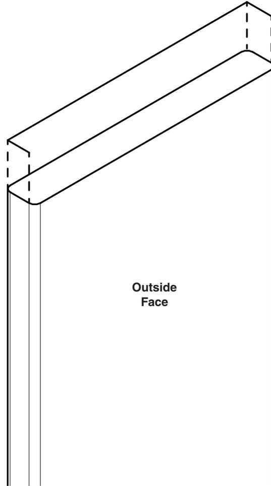
2. Remove pilaster and position "L" bracket(s) accordingly.
