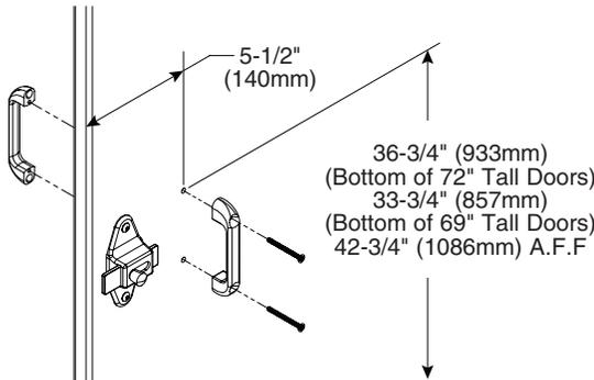
4. Position the coat hook 36" (914mm) above finished floor (hook goes on the inside of compartment). Using the hook as a template, drill (2)  $\text{Ø}7/32$ " pilot holes, 3/4" (19mm) deep. Secure with the #14 x 3/4" screws provided.
