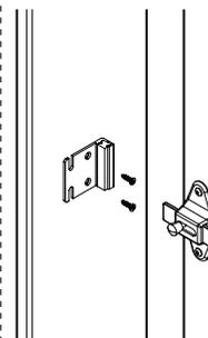
5. With the door in the closed position, place flat strike/keeper so the latch slide bar fits within the top notch.
