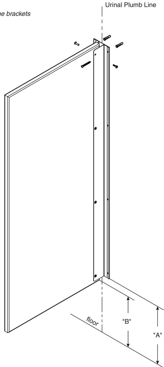
3. Insert plastic anchors in all holes and secure bracket to the wall with the #14 x 2" screws provided.
