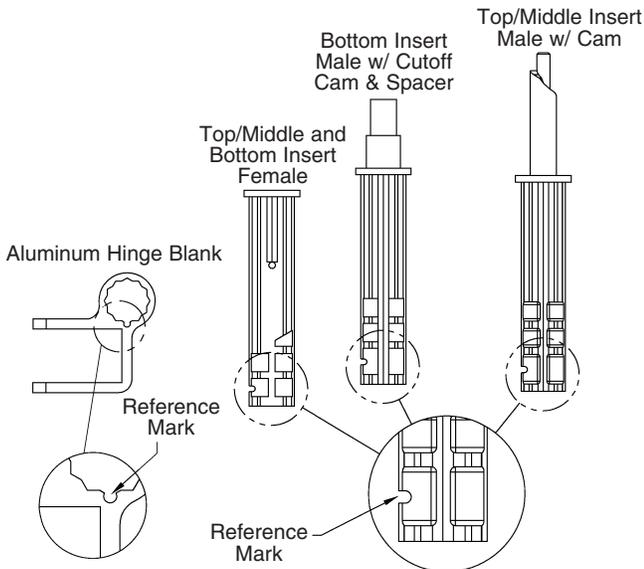
4. Assemble inserts into the hinge blanks making sure the insert collar fits tightly against each of the hinge blanks.
