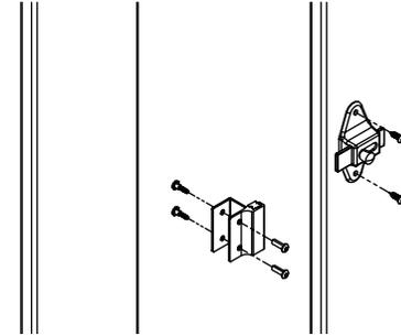
2. With the door in the closed position, place the strike/keeper on the pilaster and align the top so it is 1/4" (6mm) above the bottom of the latch slide bar. Using the strike/keeper as a template, mark the hole locations and drill  $\text{Ø}1/4$ " holes through the pilaster. Secure the strike/keeper to the pilaster with the #10-24 x 3/4" barrel nuts and #10-24 x 3/4" shoulder screws provided.
