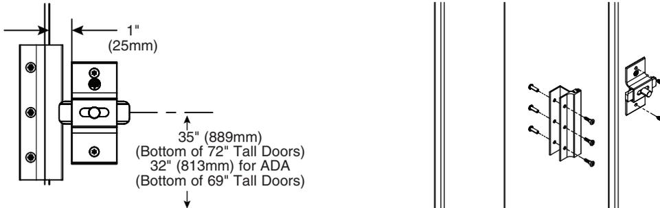
**B** With the door in the closed position, place the strike/keeper on the pilaster so it is centered on the latch slide bar. Using the strike/keeper as a template, mark the hole locations and drill Ø1/4" holes through the pilaster. Secure the strike/keeper to the pilaster with the #10-24 x 3/4" barrel nuts and #10-24 x 3/4" shoulder screws provided.
