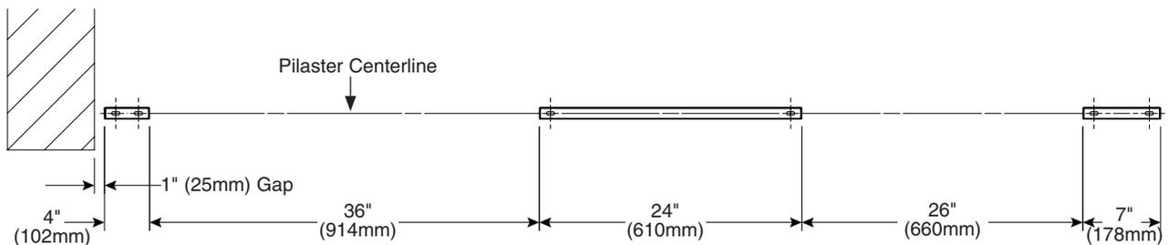
2. Using the shoe as a template, mark the hole locations on the floor. Remove the shoe and drill  $\text{\O}5/16"$  holes (min 2" [51mm] deep) into the floor. Make sure the holes are free of dirt and debris.
