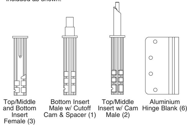
2. Find the hinge assembly that coincides with the door swing. Arrange the hinge sets as shown.
