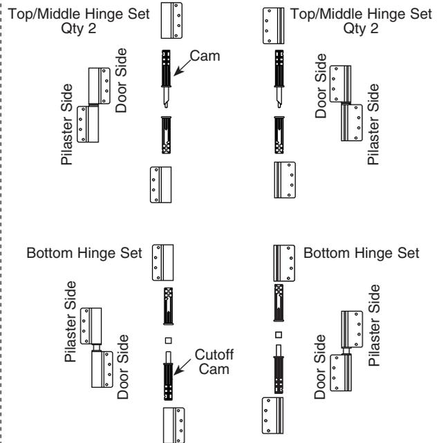
3. Align the reference marks of the inserts and hinge blanks as shown.
