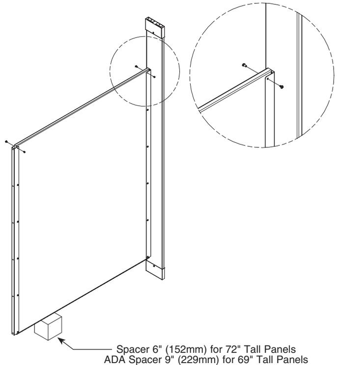
4. Using the bracket as a template, drill  $\text{\O}1/4$ " holes through the panel at each panel bracket hole. Secure the panel to the bracket using the #10-24 x 3/4" barrel nuts and #10-24 x 3/4" shoulder screws provided.
