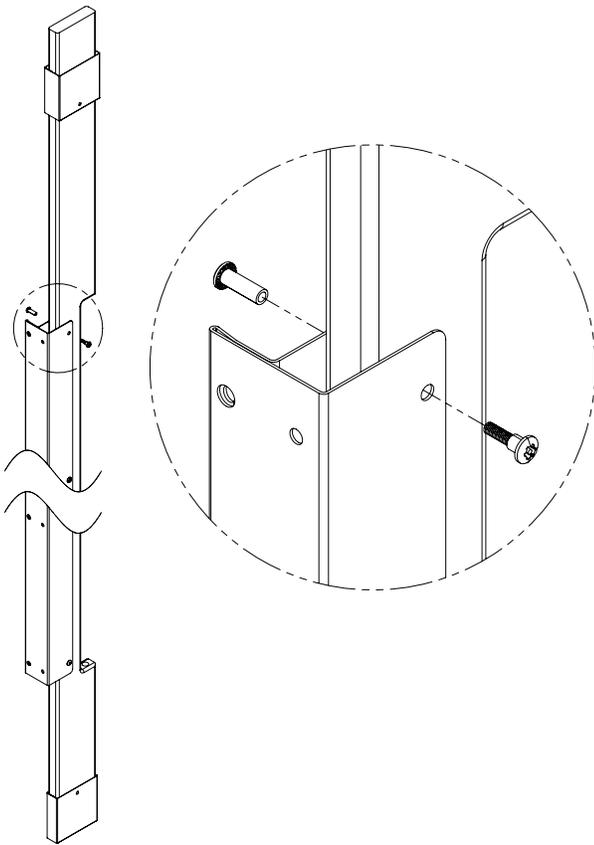
3. Using the bracket as a template, drill  $\text{\O}1/4$ " holes through the pilaster at each pilaster bracket hole. Secure the pilaster to the bracket using the #10-24 x 3/4" barrel nuts and #10-24 x 3/4" shoulder screws provided.
