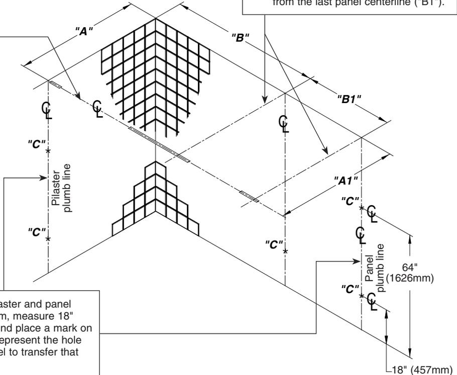
**C** Draw a plumb line on all walls from each pilaster and panel centerline. From the highest point in the room, measure 18" (457mm) and 64" (1626mm) from the floor and place a mark on the pilaster/panel plumb line. These marks represent the hole center line of the stirrup brackets. Use a level to transfer that mark to all other plumb lines ("C").
