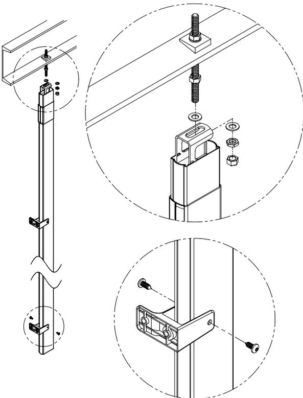
**C** Using the bracket as a template, drill Ø3/16" holes through the pilaster at each pilaster bracket hole. Secure the pilaster to the bracket using the #14 x 5/8" screws provided.
