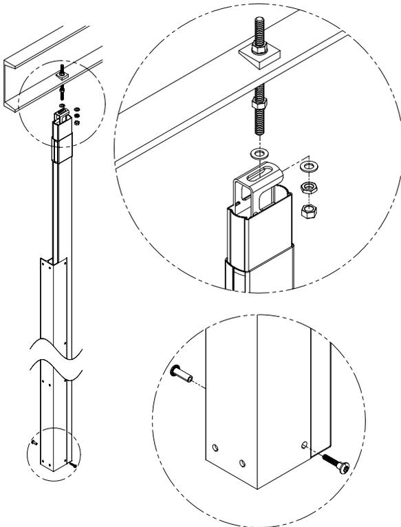
**C** Using the bracket as a template, drill Ø1/4" holes through the pilaster at each pilaster bracket hole. Secure the pilaster to the bracket using the #10-24 x 3/4" stainless barrel nuts and #10-24 x 1" stainless shoulder screws provided.
