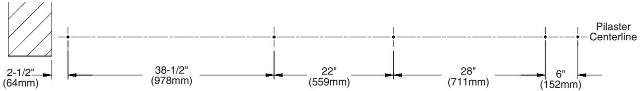
**B** Drill  $\text{Ø}3/8$ " holes in the "C" channel for each pilaster anchor required.
