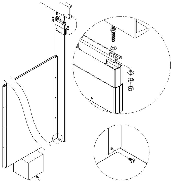
**D** Using the bracket as a template, drill Ø3/16" holes through the panel at each panel bracket hole. Secure the panel to the bracket using the #14 x 5/8" stainless screws provided.
