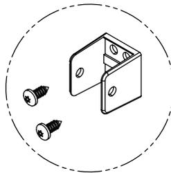
**C** Secure the stirrup brackets to the pilasters using the #14 x 5/8" screws provided.
