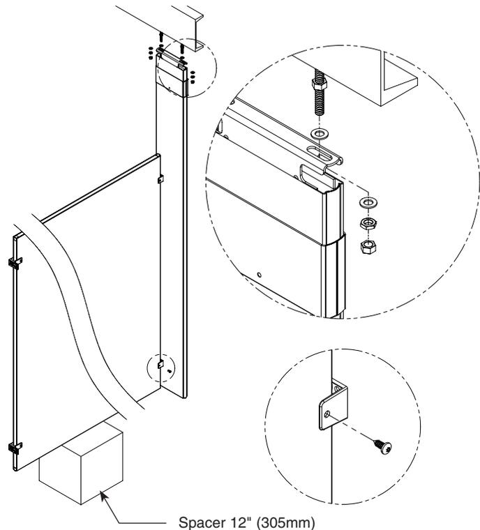
**D** Using the bracket as a template, drill Ø3/16" holes through the panel at each panel bracket hole. Secure the panel to the bracket using the #14 x 5/8" screws provided.
