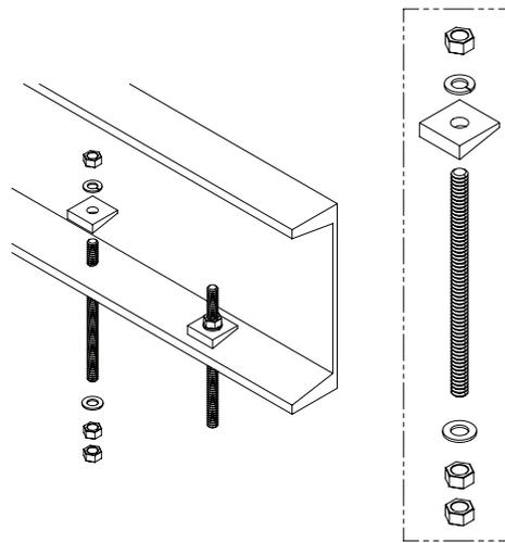
**E** From the highest point in the room, adjust the support nut to approximately 7/8" (22mm) down from the finished ceiling. Level and adjust the remaining support nuts to this height.
