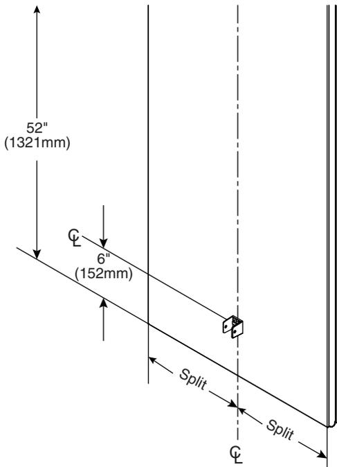
**A** Measure 6" (152mm) and 52" (1321mm) up from the bottom of each pilaster and place a mark on the pilaster split centerline.
