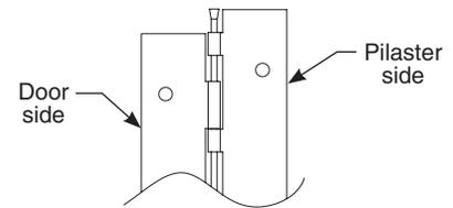
**A** Place a door on a 12" (305mm) spacer and set the door gaps. Standard hinge side gap is 9/32" (7mm).
