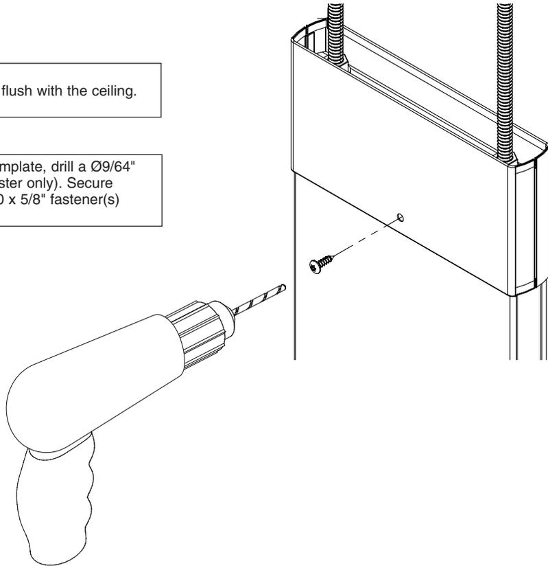
**7 Cross Bracing (Standard on Ceiling Heights 9'-0" and Above)**
