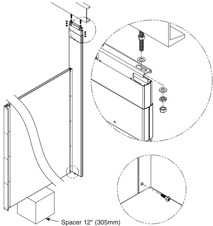
**D** Using the bracket as a template, drill Ø1/4" holes through the panel at each panel bracket hole. Secure the panel to the bracket using the #10-24 x 3/4" stainless barrel nuts and #10-24 x 3/4" stainless shoulder screws provided.
