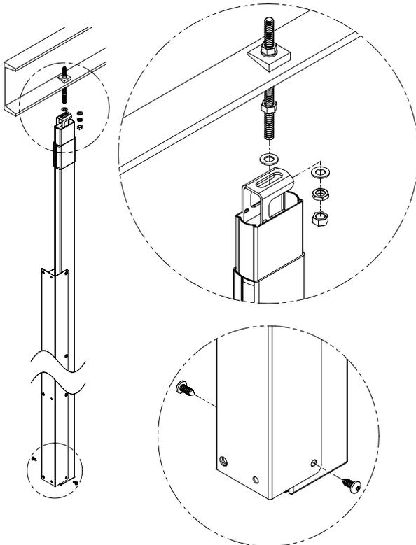
**C** Using the bracket as a template, drill Ø3/16" holes through the pilaster at each pilaster bracket hole. Secure the pilaster to the bracket using the #14 x 5/8" stainless screws provided.
