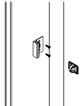
**E** Position the coat hook 36" (914mm) above finished floor (hook goes on the inside of compartment). Using the hook as a template, drill (2)  $\text{Ø}3/16$ " pilot holes through inside face of the pilaster only and secure with the #14 x 5/8" screws provided.
