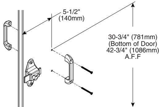
**D** Place the coat hook 3" (76mm) down from the top and 3" (76mm) from the latch side of the door (hook goes on the inside face of the door). Using the coat hook as a template, drill (2) Ø9/64" pilot holes through inside face of the door only. Secure the coat hook with the #10 x 5/8" screws provided.
