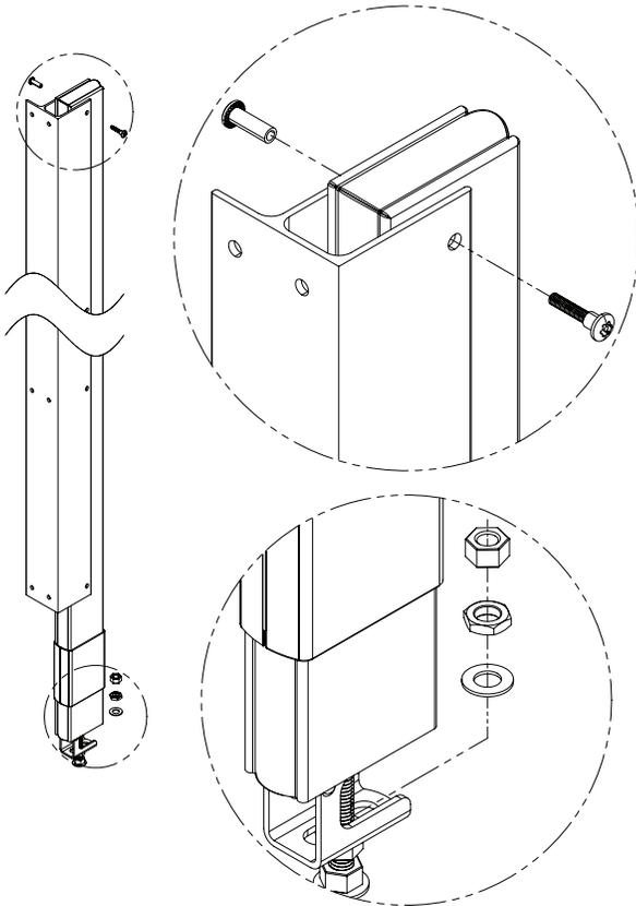
**C** Using the bracket as a template, drill Ø1/4" holes through the pilaster at each pilaster bracket hole. Secure the pilaster to the bracket using the #10-24 x 3/4" stainless barrel nuts and #10-24 x 1" stainless shoulder screws provided.
