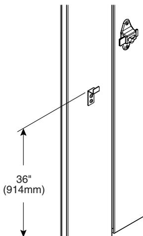
**E** Position the coat hook 36" (914mm) above finished floor (hook goes on the inside of compartment). Using the hook as a template, drill (2)  $\text{Ø}3/16"$  pilot holes through inside face of the pilaster only and secure with the #14 x 5/8" screws provided.
