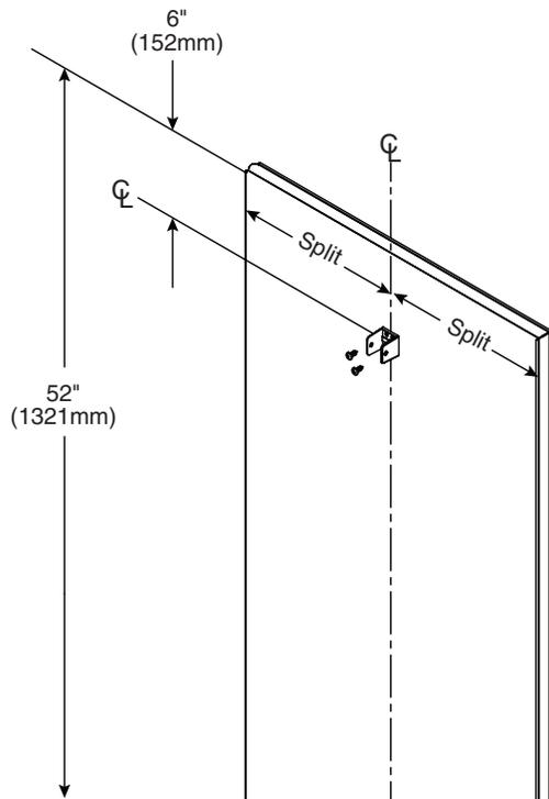
**A** Measure 6" (152mm) and 52" (1321mm) down from the top of each pilaster and place a mark on the pilaster split centerline.
