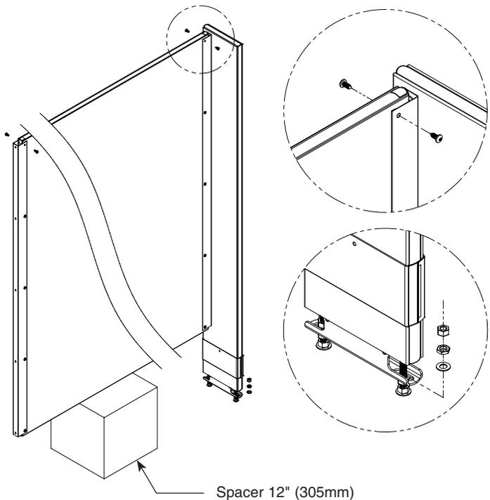
**D** Using the bracket as a template, drill Ø3/16" holes through the panel at each panel bracket hole. Secure the panel to the bracket using the #14 x 5/8" stainless screws provided.
