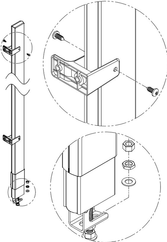
**C** Using the bracket as a template, drill Ø3/16" holes through the pilaster at each pilaster bracket hole. Secure the pilaster to the bracket using the #14 x 5/8" screws provided.
