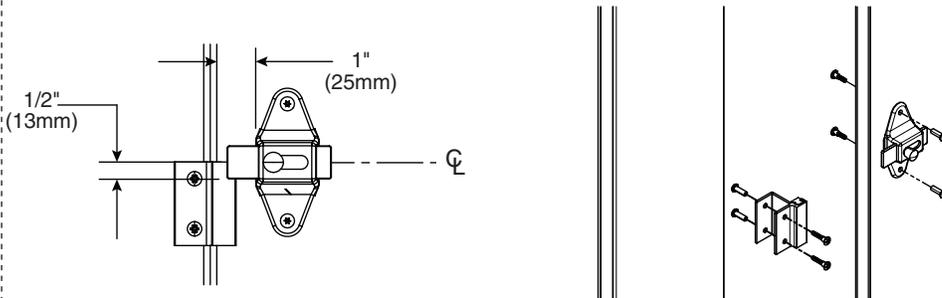
**B** With the door in the closed position, position the strike/keeper on the pilaster and align the top so it is 1/2" (13mm) above the bottom of the latch slide bar. Using the strike/keeper as a template, mark the hole locations and drill  $\text{Ø}1/4"$  holes through the pilaster. Secure the strike/keeper to the pilaster with the #10-24 x 3/4" barrel nuts and #10-24 x 1" shoulder screws provided.
