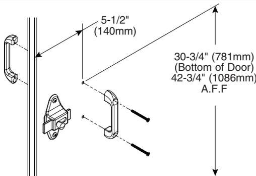
**D** Position the wall bumper 3" (76mm) up from the bottom and 3" (76mm) from the latch side of the door (bumper goes on the outside face of the door). Using the bumper as a template, drill (2)  $\text{Ø}9/64"$  pilot holes through outside face of the door only and secure to door with the #10 x 5/8" screws provided.
