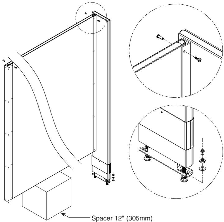
**D** Using the bracket as a template, drill Ø1/4" holes through the panel at each panel bracket hole. Secure the panel to the bracket using the #10-24 x 3/4" stainless barrel nuts and #10-24 x 3/4" stainless shoulder screws provided.
