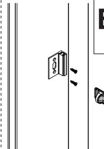
**F** Using the flat strike/keeper as a template drill (2)  $\text{Ø}1/8"$  pilot holes through one face of the pilaster only. Secure the flat strike/keeper with the #10 x 3/4" flat head screws provided.
