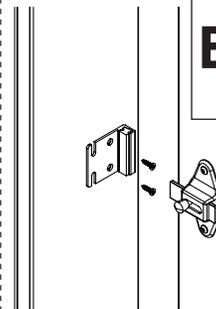
**F** Using the flat strike/keeper as a template, drill (2) Ø1/8" pilot holes through one face of the pilaster only. Secure the flat strike/keeper with the #10 x 3/4" flat head screws provided.
