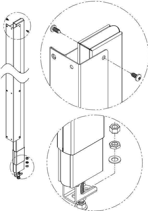
**C** Using the bracket as a template, drill Ø3/16" holes through the pilaster at each pilaster bracket hole. Secure the pilaster to the bracket using the #14 x 5/8" stainless screws provided.
