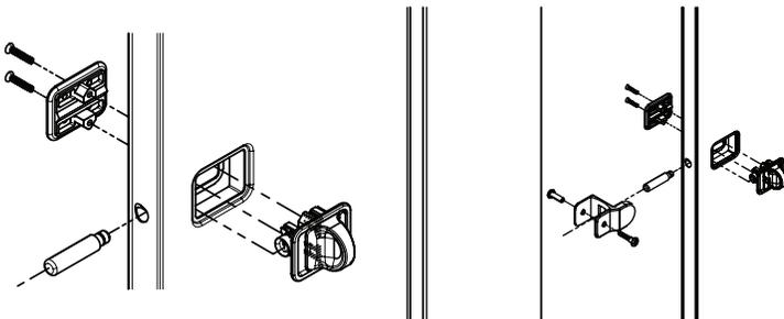
**B** Place the strike/keeper on the pilaster and center it on the opposing latch bolt. Using the strike/keeper as a template, mark the hole locations on the pilaster. Remove the strike/keeper and drill a  $\text{Ø}1/4$ " hole through the pilaster. Secure to pilaster with the #10-24 x 3/4" barrel nut and #10-24 x 1" shoulder screw provided.
