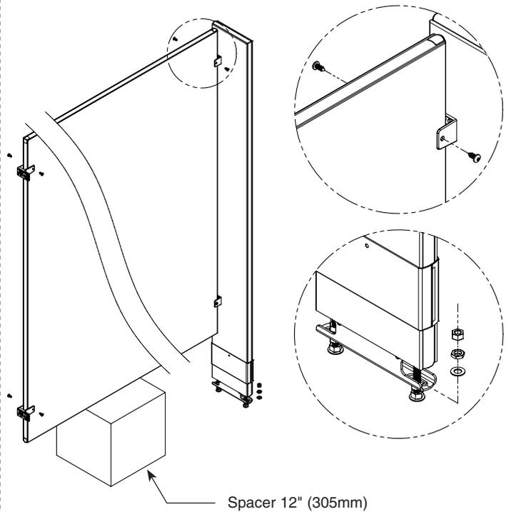
**D** Using the bracket as a template, drill Ø3/16" holes through the panel at each panel bracket hole. Secure the panel to the bracket using the #14 x 5/8" screws provided.
