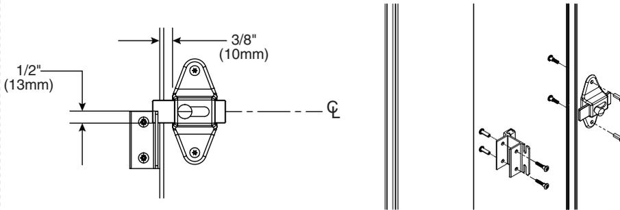
**B** With the door in the closed position, position the strike/keeper on the pilaster and align the top so it is 1/2" (13mm) above the bottom of the latch slide bar. Using the strike/keeper as a template, mark the hole locations and drill Ø1/4" holes through the pilaster. Secure the strike/keeper to the pilaster with the #10-24 x 3/4" barrel nuts and #10-24 x 1" shoulder screws provided.
