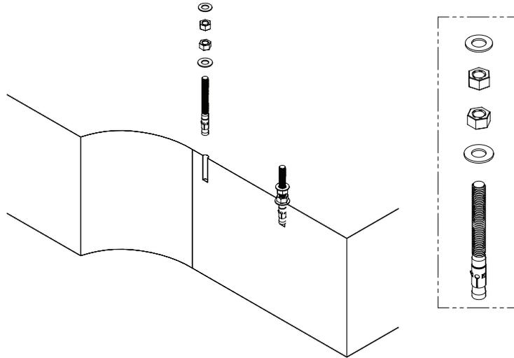
**D** From the highest point in the room, adjust the support nut and washer to approximately  $7/8$ " (22mm) above the finished floor. Level and adjust the remaining support nuts and washers to this height.
