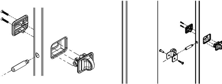
**B** Place the strike/keeper on the pilaster and center it on the opposing latch bolt. Using the strike/keeper as a template, mark the hole locations on the pilaster. Remove the strike/keeper and drill an  $\text{Ø}1/4"$  hole through the pilaster. Secure to the pilaster with the #10-24 x 3/4" barrel nut and #10-24 x 1" shoulder screw provided.
