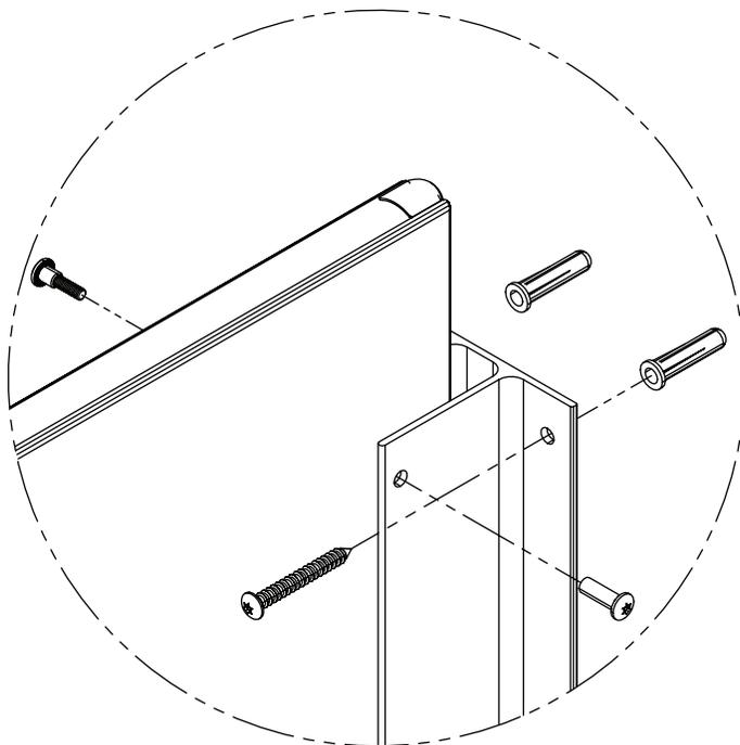
**C** Insert plastic anchors in all holes and secure bracket to the wall with the #14 x 2" stainless screws provided.
