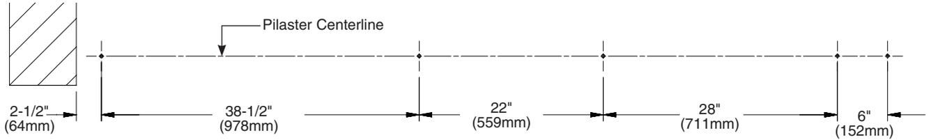
**B** Drill  $\text{Ø}3/8$ " holes (min 1-5/8" [41mm] deep) into the floor and make sure the holes are free of dirt and debris.
