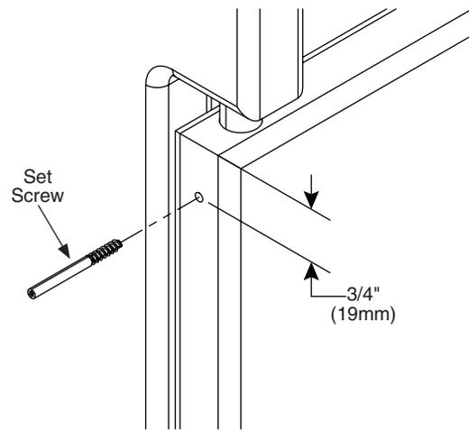
If the door is installed and pinned correctly, the door will "rise" slightly on the pintles as the door is opened.
