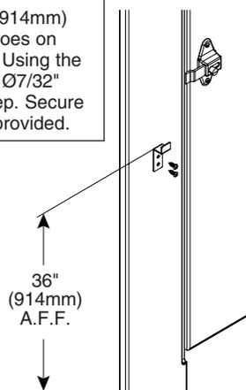
**E** Place wall bumper 3" (76mm) up from the bottom and 3" (76mm) from the "lip" of the door edge (bumper goes on the outside face of the door). Using the bumper as a template, drill (2)  $\text{\O}5/32$ " pilot holes, 3/4" (19mm) deep. Secure with the #10 x 3/4" screws provided.
