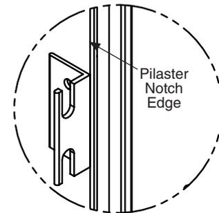
**D** Position the coat hook 36" (914mm) above finished floor (hook goes on the inside of compartment). Using the hook as a template, drill (2) Ø7/32" pilot holes, 3/4" (19mm) deep. Secure with the #14 x 3/4" screws provided.
