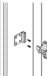
**F** Using the flat strike/keeper as a template, drill (2) Ø5/32" pilot holes, 3/4" (19mm) deep. Secure the flat strike/keeper to the pilaster using the #10 x 3/4" flat head screws provided.
