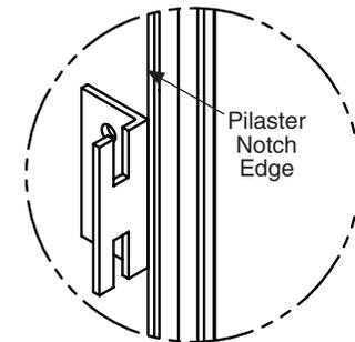
**D** Position the coat hook 36" (914mm) above finished floor (hook goes on the inside of compartment). Using the hook as a template, drill (2)  $\text{\O}7/32$ " pilot holes, 3/4" (19mm) deep. Secure with the #14 x 3/4" screws provided.
