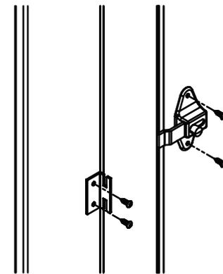
**C** For 32" - 36" doors, mark the location for the top hole on the inside face of the door 29-1/4" (743mm) up from the bottom of 55" tall doors (43-1/4" [1099mm] above finished floor) and 5-1/2" (140mm) from the "lip" of the door edge. Drill (2) Ø1/4" holes (spaced 3-1/2" [89mm] apart) through the door and secure the door pulls to the door as shown with the #10-24 x 2" flat machine screws provided.
