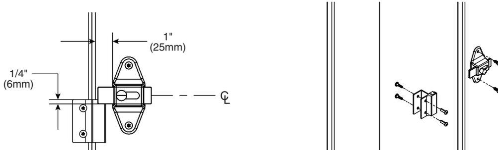
**B** With the door in the closed position, place the strike/keeper on the pilaster and align the top so it is 1/4" (6mm) above the bottom of the latch slide bar. Using the strike/keeper as a template, mark the hole locations and drill Ø1/4" holes through the pilaster. Secure the strike/keeper to the pilaster with the #10-24 x 3/4" barrel nuts and #10-24 x 3/4" shoulder screws provided.
