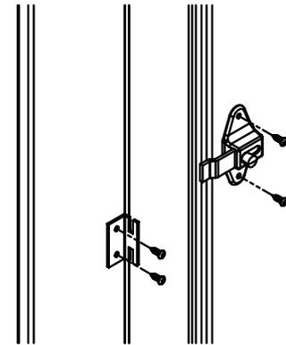
**C** Mark the location for the top hole on the inside face of the door 29-1/4" (743mm) up from the bottom of 55" tall doors (43-1/4" [1099mm] above finished floor) and 5-1/2" (140mm) from the "lip" of the door edge. Drill (2)  $\text{\O}1/4$ " holes (spaced 3-1/2" [89mm] apart) through the door and secure the door pulls to the door as shown with the #10-24 x 2" flat machine screws provided.
