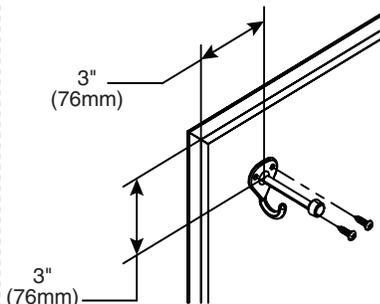
**E** With the door in the closed position, place flat strike/keeper on the pilaster and align the slot so it is centered around the latch slide bar.
