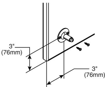
**F** With the door in the closed position, place flat strike/keeper so it is centered on the latch slide bar.
