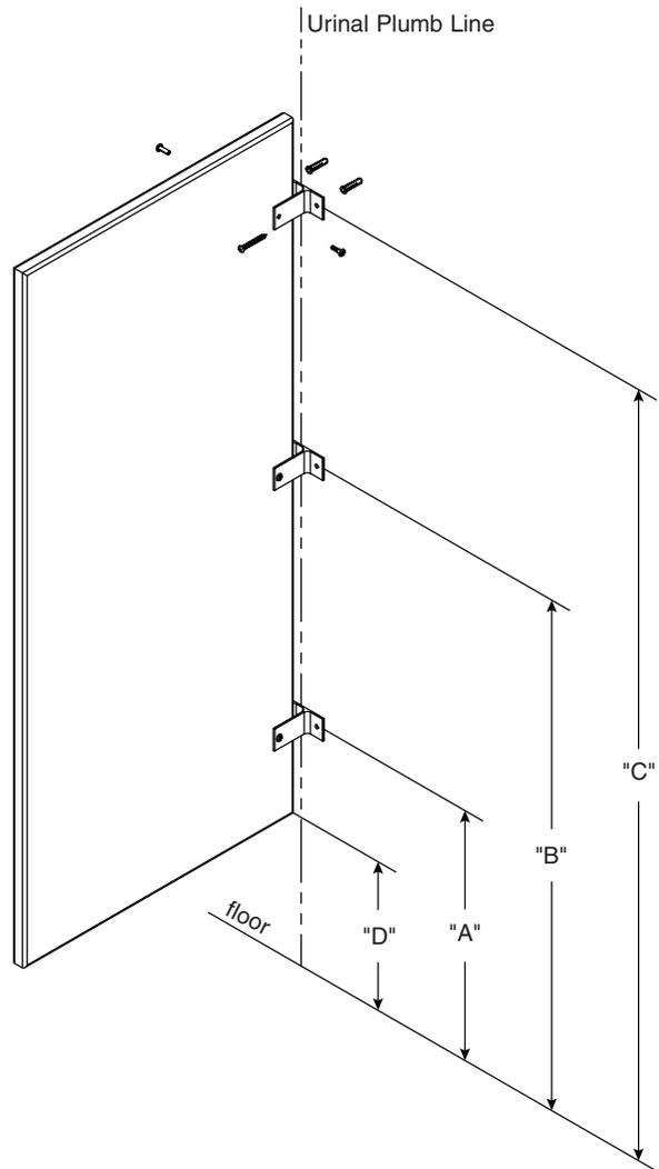
**C** Insert plastic anchors in all holes and secure bracket to the wall with the #14 x 2" screws provided.
