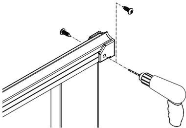
**D** Make sure the pilaster is plumb and that the spacing between the pilasters for the doors is the correct dimension. On the back of each pilaster (starting with the first pilaster), drill a Ø7/32" hole through one face of the headrail only.
