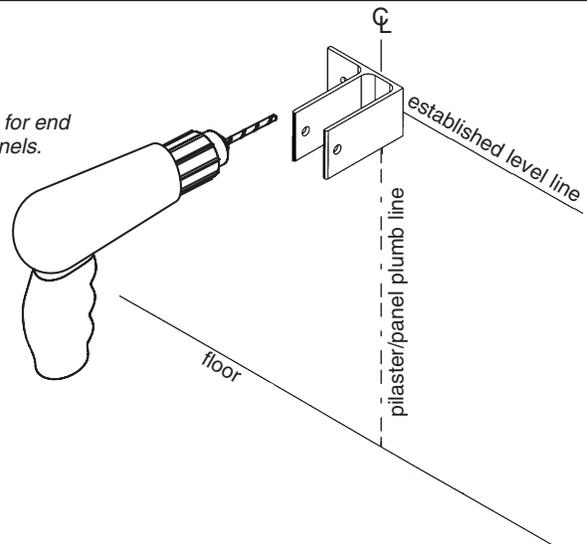
**A** Place the center of each stirrup bracket at the established level line. Center the bracket opening on the pilaster/panel plumb line.
