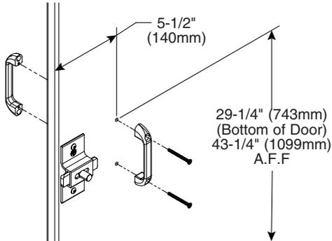
**D** Place coat hook 3" (76mm) down from the top and 3" (76mm) from the latch side of the door (hook goes on the inside face of the door). Using the hook as a template, drill (2) Ø5/32" pilot holes, 3/4" (19mm) deep. Secure with the #10 x 3/4" screws provided.
