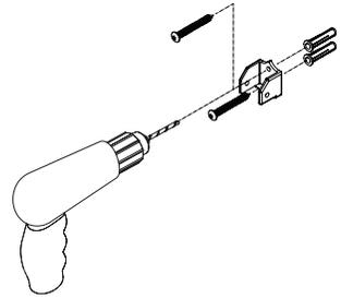
**C** Place headrail over the top of the pilasters and slide it tight into the mounting bracket. Use the mounting bracket as a template and drill a Ø7/32" hole through the headrail. Secure the headrail to the mounting bracket with the #10 x 5/8" screws provided.
