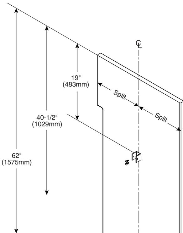
**A** Measure 19" (483mm), 40-1/2" (1029mm), and 62" (1575mm) down from the top of each pilaster and place a mark on the pilaster split centerline.
