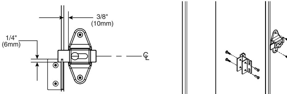
**B** With the door in the closed position, place the strike/keeper on the pilaster and align the top so it is 1/4" (6mm) above the bottom of the latch slide bar. Using the strike/keeper as a template, mark the hole locations and drill Ø1/4" holes through the pilaster. Secure the strike/keeper to the pilaster with the #10-24 x 3/4" barrel nuts and #10-24 x 3/4" shoulder screws provided.
