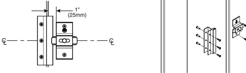
**B** With the door in the closed position, place the strike/keeper on the pilaster so it is centered on the latch slide bar. Using the strike/keeper as a template, mark the hole locations and drill Ø1/4" holes through the pilaster. Secure the strike/keeper to the pilaster with the #10-24 x 3/4" barrel nuts and #10-24 x 3/4" shoulder screws provided.
