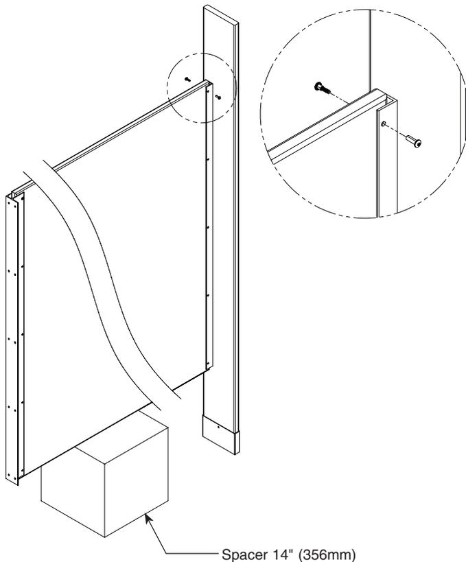
**6b Pilasters and Panels with Stirrup Brackets (Optional)**
