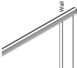
**B** Place the headrail bracket on the outline marked on the wall and mark the locations of the mounting holes. Remove bracket and drill (2) Ø5/16" holes at a minimum of 2" (51mm) deep. Prior to securing to the wall, enlarge the (2) back mounting holes of the bracket to Ø1/4". Secure the bracket to the wall with the #14 x 2" screws and plastic anchors provided.
