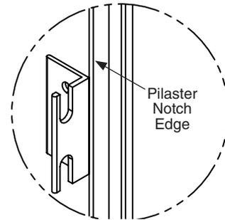
**D** Place the coat hook 3" (76mm) down from the top and 3" (76mm) from the "lip" of the door edge (hook goes on the inside face of the door). Using the hook as a template, drill (2) Ø5/32" pilot holes, 3/4" (19mm) deep. Secure with the #10 x 3/4" screws provided.
