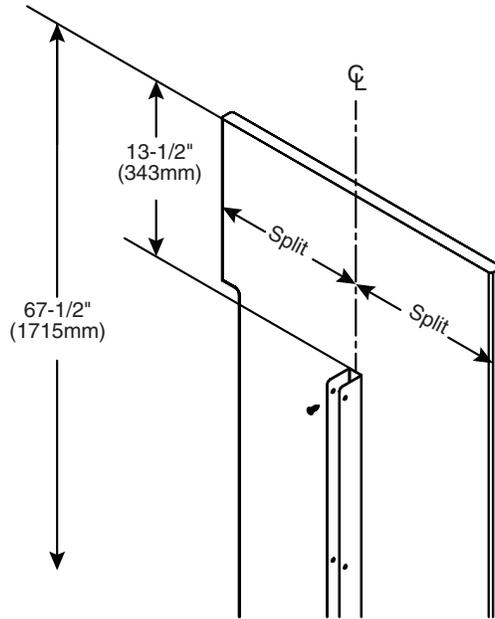
**A** Measure 13-1/2" (343mm) and 67-1/2" (1715mm) down from the top of each pilaster and place a mark on the pilaster split centerline.
