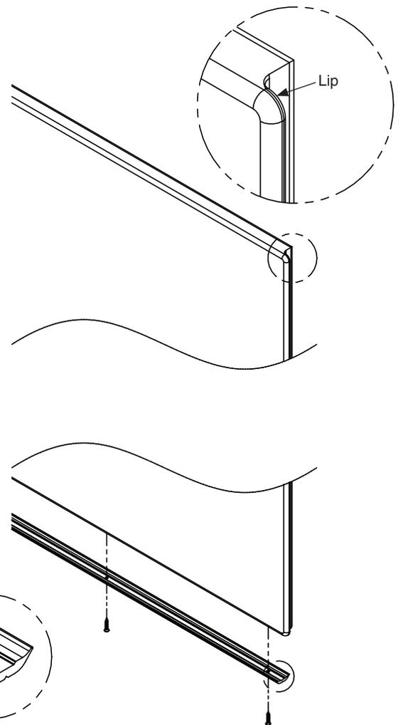
**9b Continuous Spring-Loaded Piano Hinge - Stainless Steel (Optional)**
