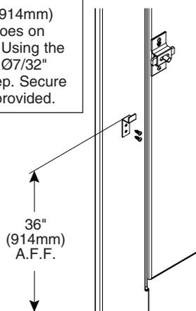
**E** Place wall bumper 3" (76mm) up from the bottom and 3" (76mm) from the "lip" of the door edge (bumper goes on the outside face of the door). Using the bumper as a template, drill (2) Ø5/32" pilot holes, 3/4" (19mm) deep. Secure with the #10 x 3/4" screws provided.
