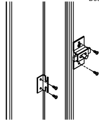
**C** Mark the location for the top hole on the inside face of the door 29-1/4" (743mm) up from the bottom of 55" tall doors (43-1/4" [1099mm] above finished floor) and 5-1/2" (140mm) from the "lip" of the door edge. Drill (2) Ø1/4" holes (spaced 3-1/2" [89mm] apart) through the door and secure the door pulls to the door as shown with the #10-24 x 2" flat machine screws provided.
