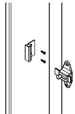
**G** Using the flat strike/keeper as a template, drill (2) Ø5/32" pilot holes, 3/4" (19mm) deep. Secure the flat strike/keeper to the pilaster using the #10 x 3/4" flat head screws provided.
