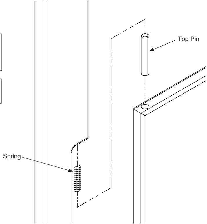
**G** With the door in the desired "at rest" position, measure approximately 3" (76mm) down from the pilaster cutout and place a mark centered on the pilaster edge.
