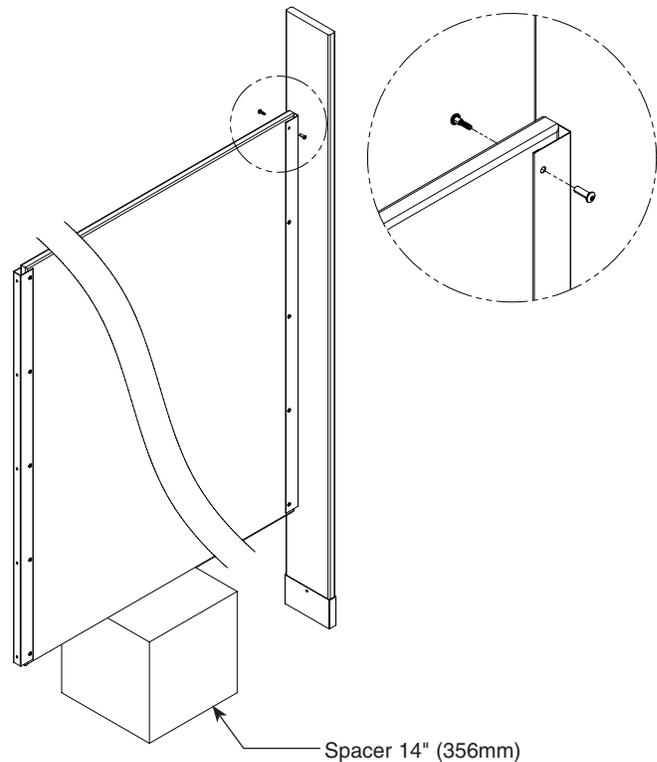
**6a Pilasters and Panels with Aluminum Continuous Brackets (Optional)**
