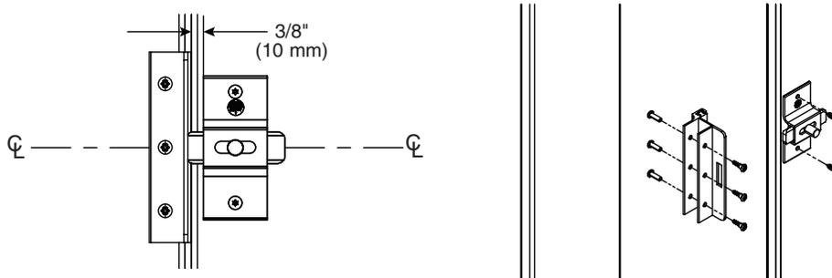
**B** With the door in the closed position, place the strike/keeper on the pilaster and align the slot so it is centered around the latch slide bar. Using the strike/keeper as a template, mark the hole locations and drill Ø1/4" holes through the pilaster. Secure the strike/keeper to the pilaster with the #10-24 x 3/4" barrel nuts and #10-24 x 3/4" shoulder screws provided.
