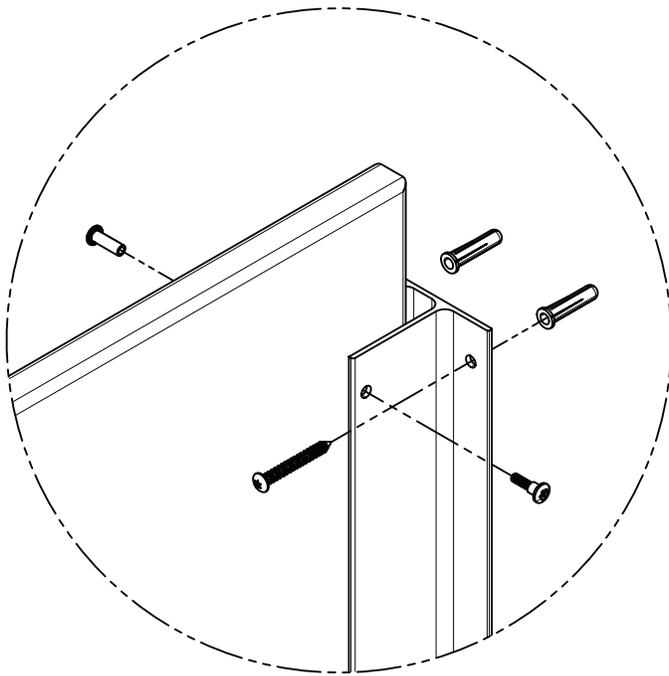
**C** Insert plastic anchors in all holes and secure bracket to the wall with the #14 x 2" screws provided.
