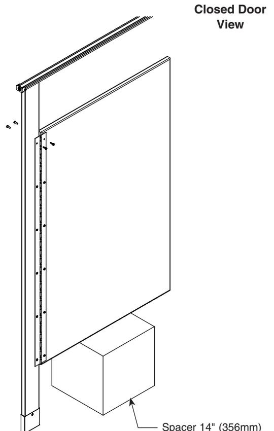
**9c Continuous Spring-Loaded Piano Hinge - Aluminum (Optional)**
